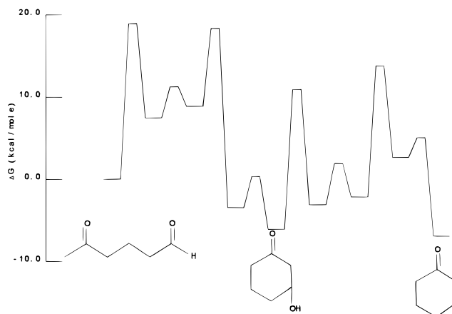
Figure 4. Reaction coordinate diagram for the aldol condensation of 5-oxohexanal. See legend to Figure 1.
