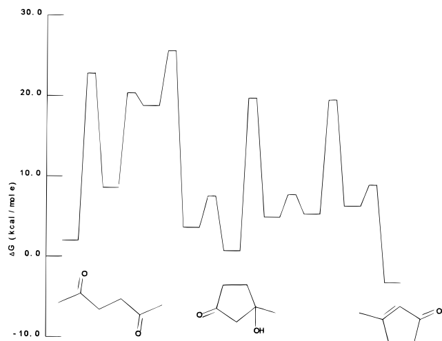
Figure 1. Reaction coordinate diagram for the aldol condensation of 2,5-hexanedione. The steps shown are as follows: ketone to enolate; enolate to reactive conformation (rate constant in the thermodynamically favored direction assumed to have k = 10^{11} \text{ s}^{-1} ); reactive conformation to ketol alkoxide; ketol alkoxide to ketol (assumed to have k = 10^{10} \text{ s}^{-1} ); ketol to enolate; enolate to reactive conformation (rate constant in the thermodynamically favored direction assumed to have k = 10^{11} \text{ s}^{-1} ); reactive conformation to encounter complex with hydroxide; diffusional separation of hydroxide (assumed to have k = 10^{11} \text{ s}^{-1} ).
